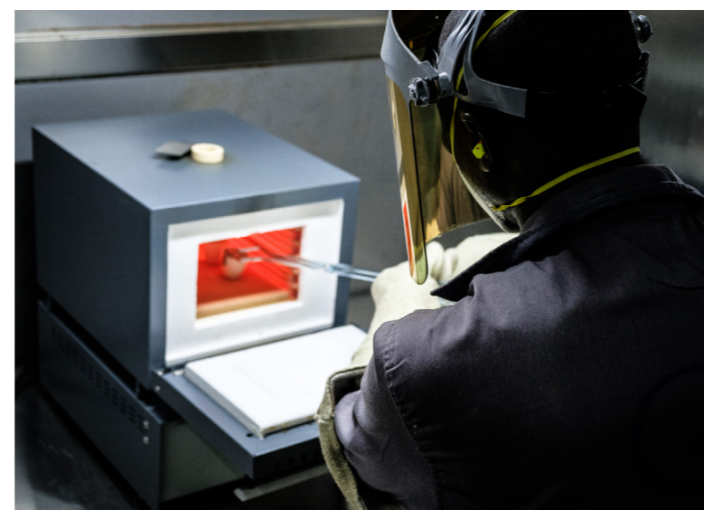
Loss on Ignition (LOI) test to analyse Graphite purity
